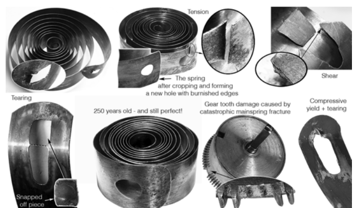
Figure 7: Just a few examples of peg and hole mainspring failure
